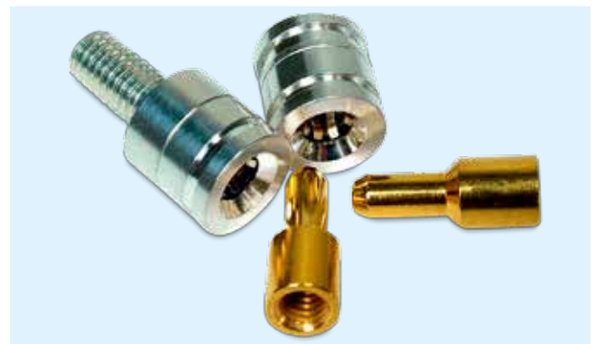
Application in the automotive sector: – Special lamella with radial compensation ( \pm 0.3 mm) – Rated current 25 A – Vibration-resistant – Application temperature -40 °C to +125 °C, briefly +170 °C
